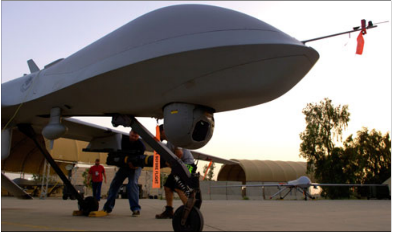
General Atomics contractors load a Hellfire missile onto an MQ-1 Predator in Iraq.
