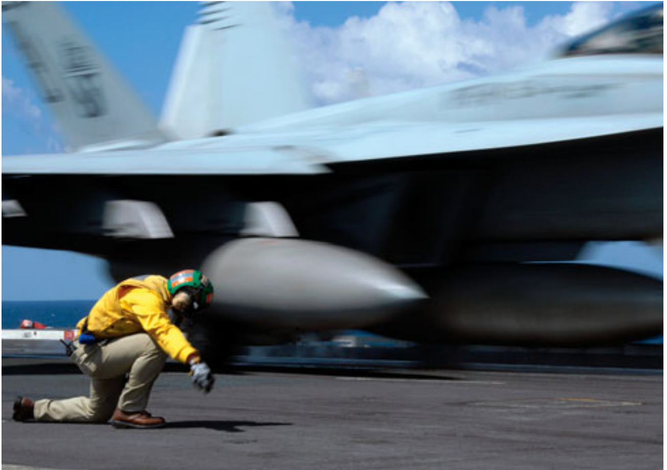
When the shear pin shears the jet is unleashed, and so is a steam catapult that hurls the plane, from 0 to 130 miles per hour in two seconds.
